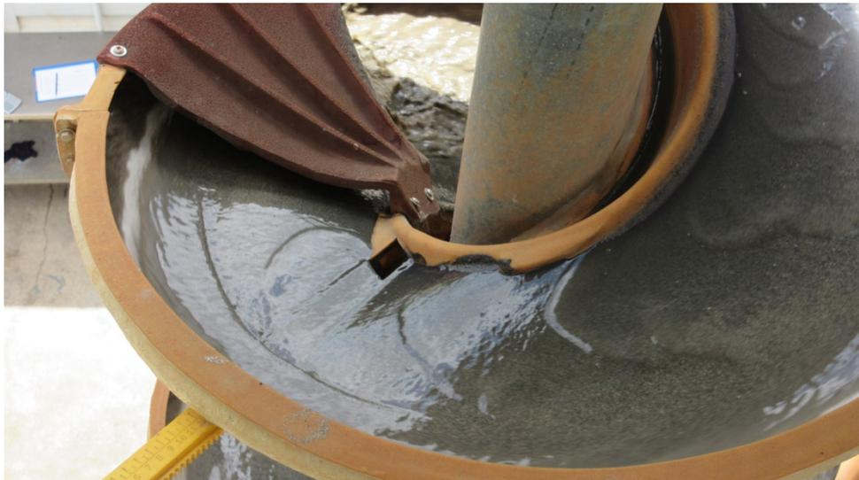
**Plate 2** – Darker heavy minerals (including magnetite) are concentrated toward the centre of the spirals, where they are separated for recovery.
