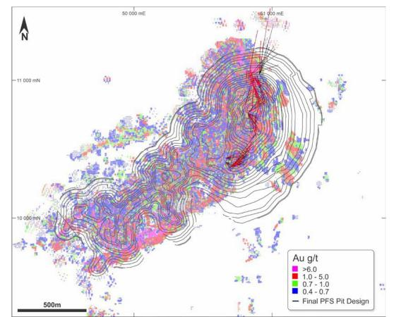
*Figure 5:* Planview projection of the KOTH resource model and Tarmoola open pit, showing the drill traces of which, the assay results are included in this report. The intercept highlights in the diagram are the intercepts that occur outside the current May 2019 release resource model.
