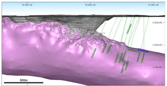
*Figure 6:* Long section through looking west, displaying drill trace of KHRD0352 (blue) and the previously announced hole KHRD0278 relative to the underground workings (grey), historical TARD holes (green) and granodiorite (pink).
