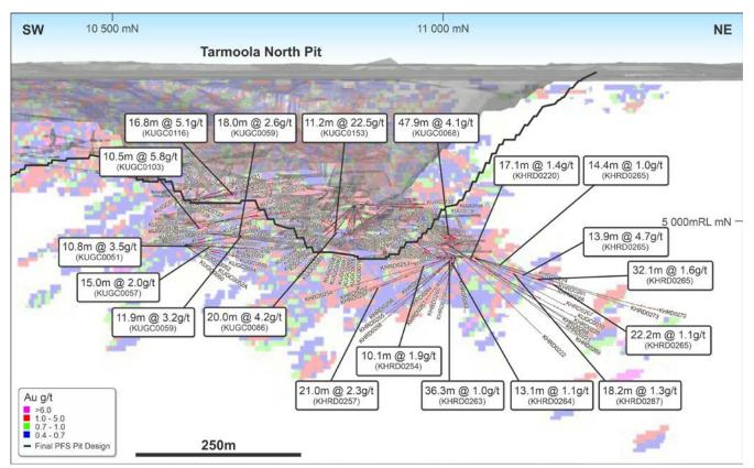
*Figure 4:* Close up Longitudinal Projection of the KOTH resource model and Tarmoola open pit showing some of the key assay results reported, looking orthogonal to strike, showing the drill traces of which, the assay results are included in this report. The intercept highlights in the diagram are the intercepts that occur outside the current May 2019 release resource model.
