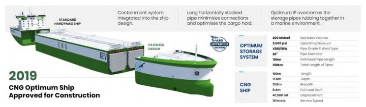
Note: The schematic of the Optimum CNG vessel presented above is indicative of the loading and unloading of CNG using onshore facilities. Modifications to the ship will be made for offshore loading systems such as a STL or SAL system, however it does not require further approvals from ABS for the Optimum CNG containment system.
